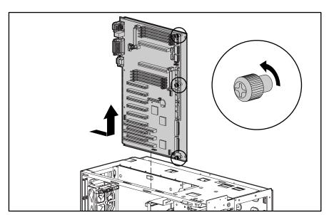
Figure 2-37. Removing the system I/O board with subpan
